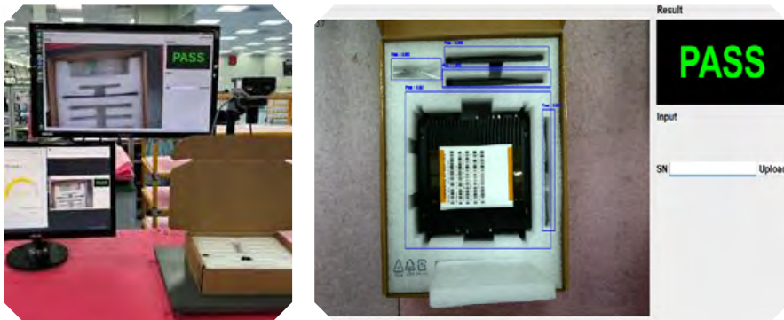
▲ The efficiency of accessory inspections has been increased through the use of AVI technology.
